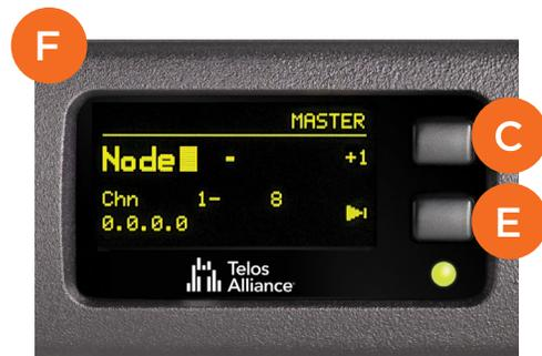
7. After the ID number is chosen, press the bottom button (E) once more to save the ID. The xNode's IP address and channel numbers are automatically assigned based on the ID number, and are displayed on the OLED (G).
